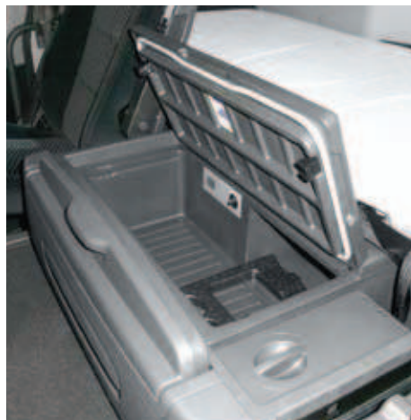
Shown as built-in solution: Dometic cooler for Actros MP2/MP3
