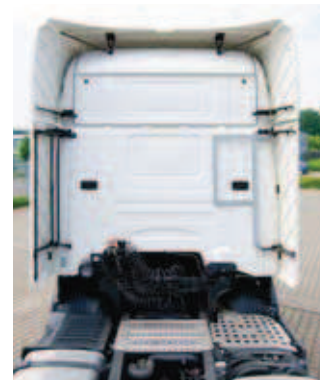
Scania fastening frame SCAN1 SP900
