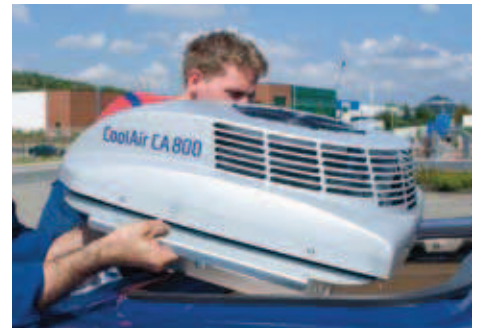
Use existing mounting holes when fitting the new roof air conditioner
