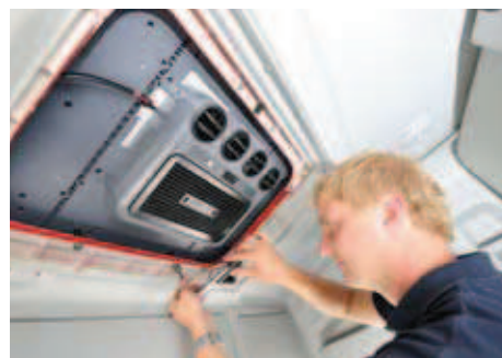
Custom-made for Iveco Stralis: the CA 850S replaces the roof window
