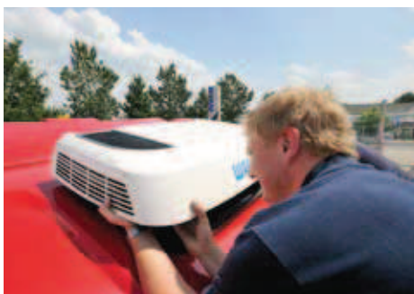
Final finishing touches: fitting the new roof air conditioner
